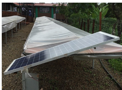
Figure 3 - Mango fruits processed in a tunnel solar dryer
