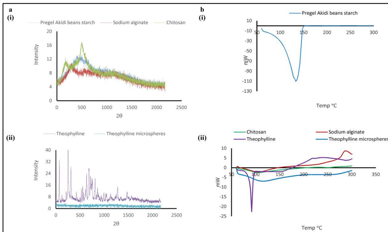
**Figure 4:** (a) X-ray diffraction (XRD) spectra of (i) pregelatinized Akidi beans starch, chitosan, sodium alginate, (ii) theophylline and theophylline microspheres, (b) Differential Scanning Calorimetry (DSC) of (i) pregelatinized Akidi beans starch, chitosan, (ii) sodium alginate, theophylline and theophylline microspheres
