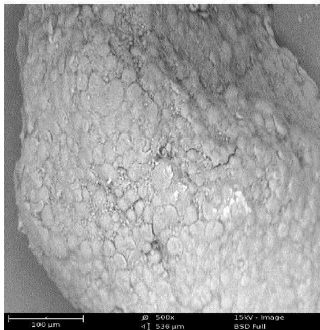
**Figure 2: Scanning electron micrographs (SEM) of pregelatinized Akidi beans starch.**
