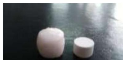
Figure 4: Photograph of batch F8 acyclovir floating tablets in the dry (right) and wetted (left) state after eight hours in 0.1N HCl.
