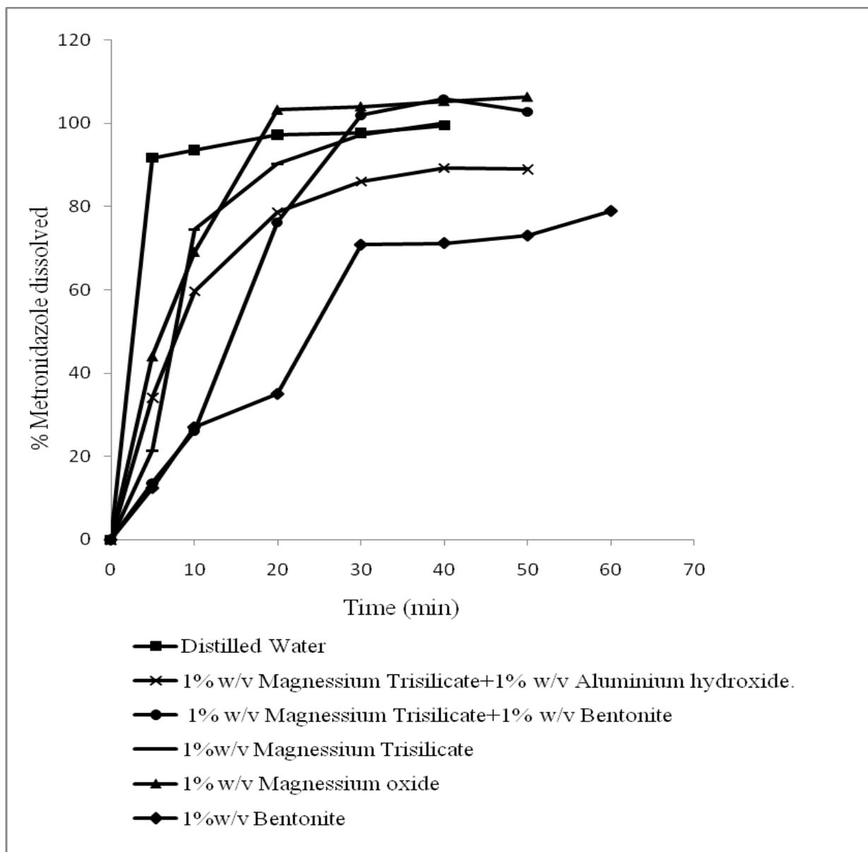
**Figure 2.** The effect of antacid on the dissolution profile of metronidazole from tablets in various media at  $37 \pm 0.5$  °C.
