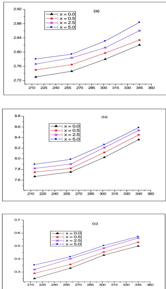
Figure 4. (a) Refractive index, (b) Real part of dielectric constant, and (c) Imaginary part of dielectric constant against film thickness at different antimony concentrations;  $\lambda = 700\text{nm}$
