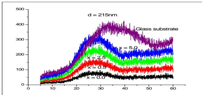
Figure 1. X-Ray Diffraction pattern for a 215nm thin films
