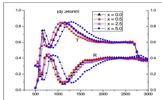
Figure 2. Transmittance and Reflectance against wavelength (nm) at different film thicknesses: (a) 215nm, (b) 260nm, (c) 302nm, and (d) 345nm
