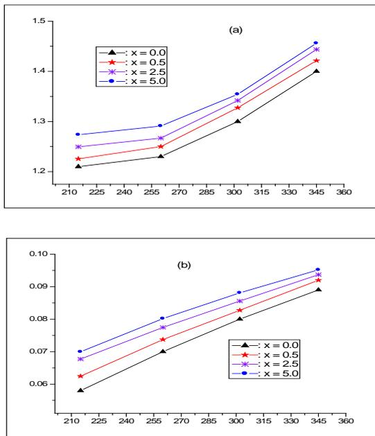
Figure 3. (a) Absorption coefficient and (b) Extinction coefficient against film thickness at different atomic percentages of antimony;  $\lambda = 700\text{nm}$
