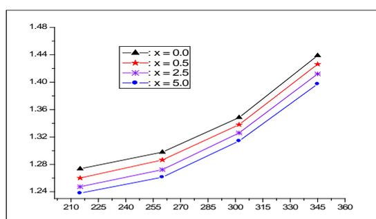
Figure 5. Energy band gap (eV) against film thickness (nm) at different antimony concentration;  $\lambda = 700\text{nm}$
