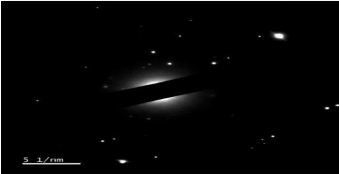
**Figure 8d:** Selected Area Electron Diffraction pattern image of coupled titanium dioxide coupled with molybdenum trioxide nanocomposite
