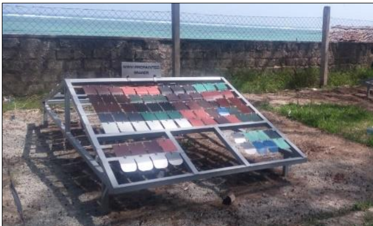
Figure 2: A set-up for outdoor exposure of pre-painted metallic coated sheets at Diani site
