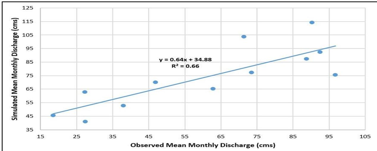
Figure 5: Correlation of mean monthly observed and simulated water yields (cms) at Kiptiget RGS
