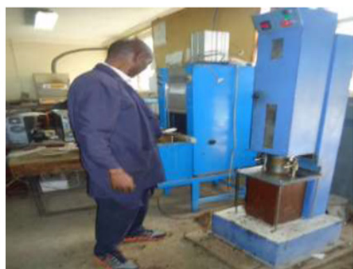
d) Marshall Compacting at 75 blows
