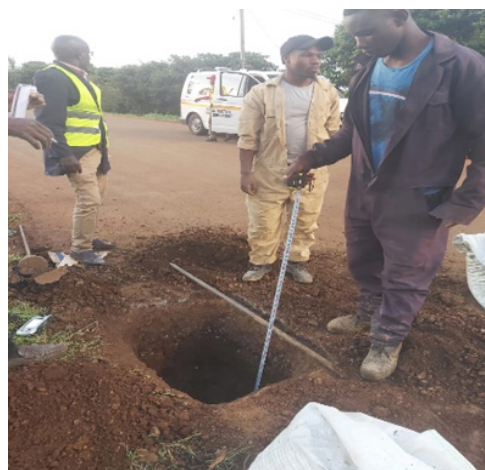
b) Layer thickness measurement
