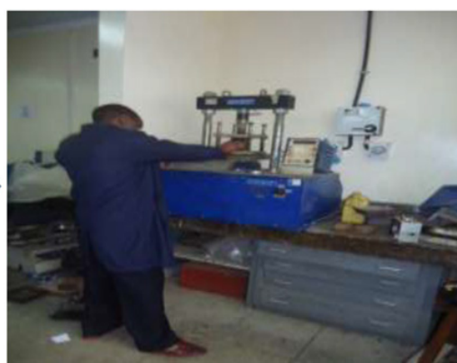
f) ITS testing using Multi-Speed Tester
