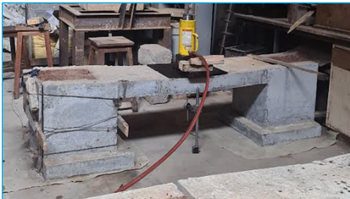
FIGURE 9 Failed integral bridge model Source: Author, 2024
