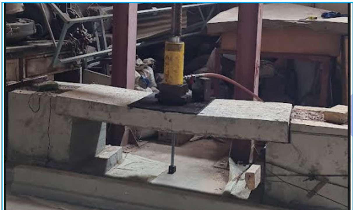
FIGURE 8 Failed Non-integral bridge model Source: Author, 2024
