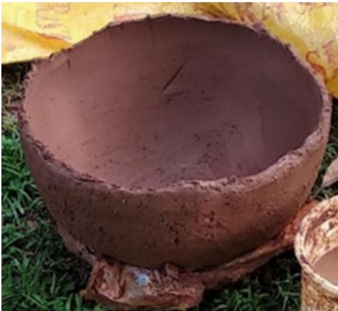
FIGURE 1c Part of the clay cooking stove in leather hard stage Source: Author 2020
