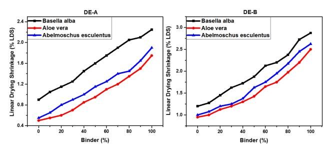
Figure 1: Variation of linear drying shrinkage with binder content in dried DE-A and DE-B discs
