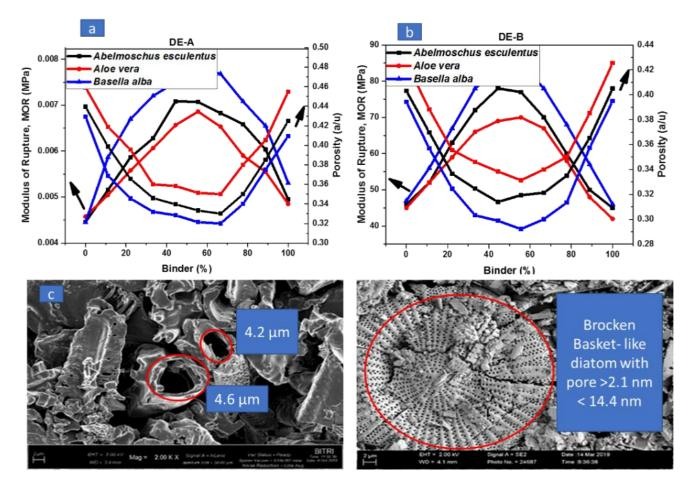
**Figure 3:** The plot of modulus of rupture against binder concentration used to fabricate diatomaceous earth A (a) and B (b) membranes fired at 950.0 °C and their micrograph
