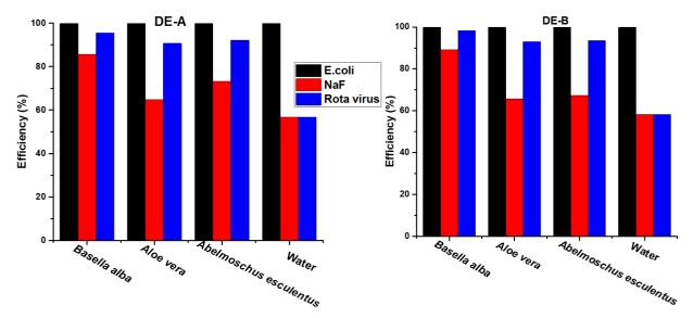
**Figure 4:** The bar chart of the percentage efficiency of the membrane fabricated with diatomaceous earth (DE-A and DE-B) and different binders: Abelmoschus esculentus, Aloe vera, and Basella alba in filtering water contaminated with E.coli, NaF, and Rotavirus
