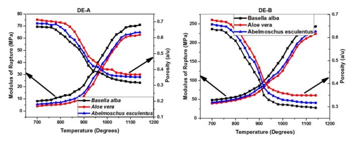
Figure 2: The plot of modulus of rapture and porosity against firing temperature of diatomaceous earth A (DE-A) and diatomaceous earth B samples (DE-B)
